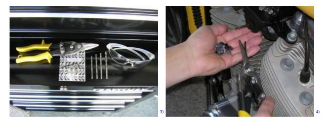
If the ID of the new knob is too small, you'll need to drill the hole out larger to go over the stud. Start with a small bit and work your way up with larger bits until it fits the rod. Note: Drilling into plastic creates heat which melts the ID larger than the drill bit.
