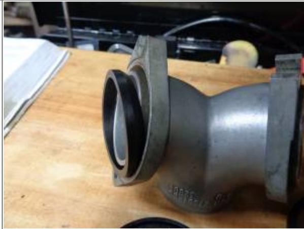
The carb seal goes on the intake port. Check that the seal is fully seated when installed. <sup>7)</sup>
