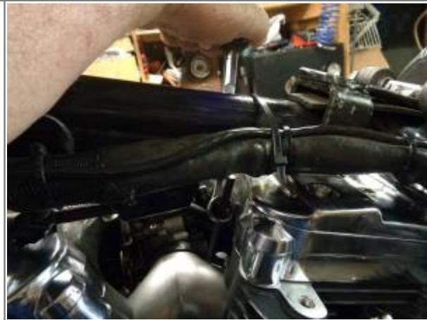
Do not over-torque the intake bolts. This will probably cause a leak.
