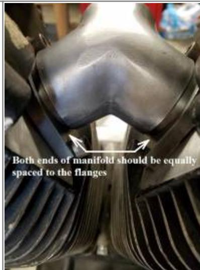
Having the carb in place allows the carb seal and the manifold to squarely mate with the carb before tightening the intake bolts.<sup>11)</sup>
