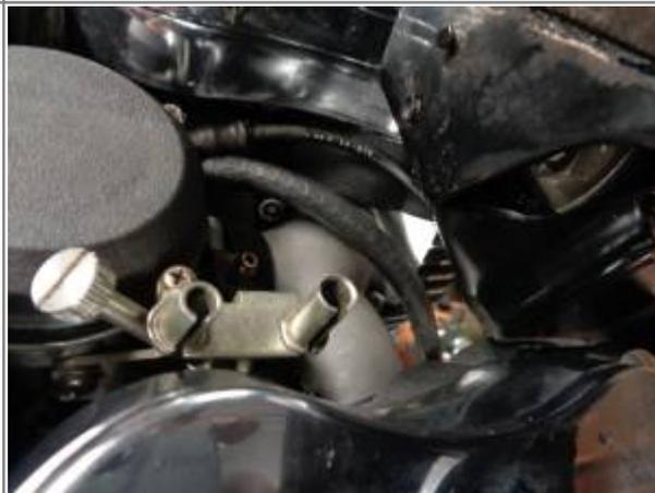
You can use a long ball type Allen wrench on the intake bolts.
