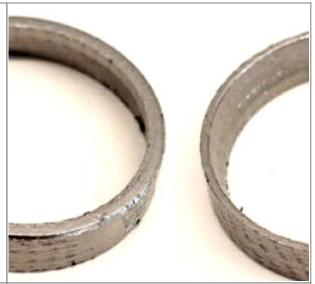
Cometic (bottom) versus HD (top) exhaust gasket comparison. 3)
