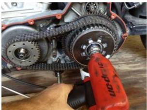
Normally when loosening or tightening these nuts, you will need to **lock the hub & sprocket** - Do not wedge the chain.
