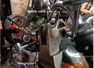
Then pull the clutch cable down thru the trees and lay it out in front of the bike.
