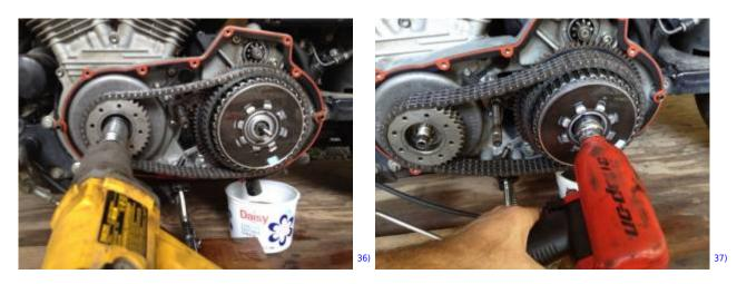
Normally when loosening or tightening these nuts, you will need to **lock the hub & sprocket** - Do not wedge the chain.
