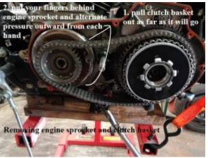
The engine sprocket and clutch hub should be removed as one unit.
