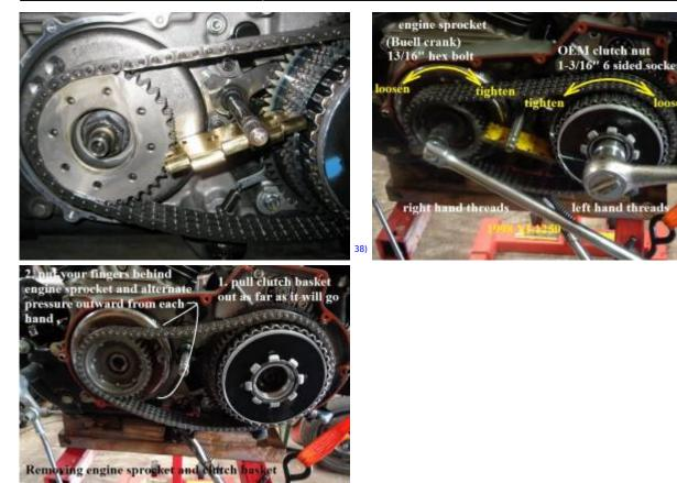
The engine sprocket and clutch hub should be removed as one unit.
