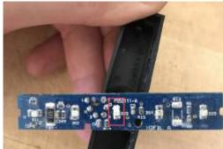
11. Next grab a new OSG5120641E Green led and test it. For the purpose of the test i assembled the scientific instrument shown below; a CR2032 flat battery, two short wires and everything held in place with a clothespin. Touching the LED's terminal should cause it to illuminate. If it does not, try reversing the polarity. LED's are polarity sensitive.
