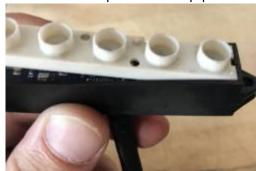
4. At this point and before disconnecting any other plugs, turn key to ignition/run position, take a multimeter and check if voltage is recorded across the Neutral LED. Cross reference it with another working LED.
