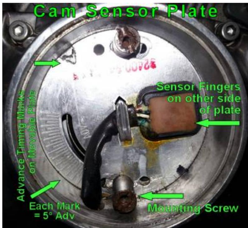
**Moving the Cam Sensor Plate Clockwise (CW) will increase the Advance Before TDC. Moving the plate Counterclockwise (CCW) will retard (or reduce) the Advance Before TDC. TAKE NOTE that each timing mark on the plate (long-to-short) is equal to changing the ignition timing by about 5°. Move the plate VERY LITTLE to make adjustments.** <sup>13)</sup>
