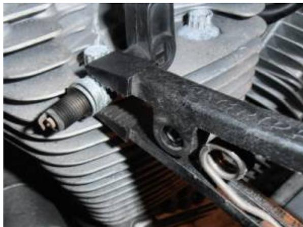
On the coil, the BLUE Wire is the trigger wire from the Ignition Control Module & the PINK Wire goes to the Tachometer. The WHITE Wire(s) are power from the Run/Stop Switch. On later version retrofit modules for 86-90, the trigger wire may be a PINK Wire, since the 1991-later connectorized stock modules used a PINK Wire for the trigger signal.
