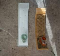
Make sure you line up the holes and push the new pickup sock on. Then put the new zip ties on and the crimp ring to hold the new pick up sock on.
