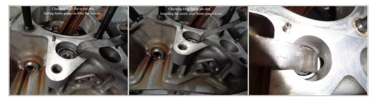
If a screw locks up a lifter when installed, the back hole did wander away from center. The lifter below was moving fine with the bolt inserted and threaded to the head but not tightened. It locked up as soon as the bolt was torqued to 10 in lbs.
