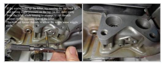
With the stock pins on a worn engine, there was a slight circular twist possible to the lifters with the pins installed.
