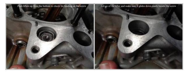
You can use a feeler gauge between the pin and lifter flat.
