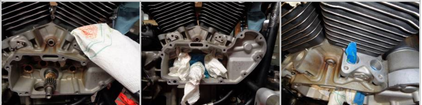
Protect the gearcase oiling holes from aluminum shavings. 17)
