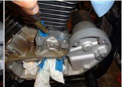
You can use a small inspection camera to check the oiling holes for aluminum shavings. 23 This is the new extended pin hole. 24)
