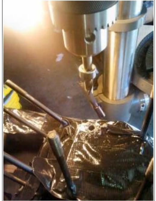
Once the hole is drilled with the X Bit, then you use the counter bore bit, it has a built in stop so you can't go to far.
