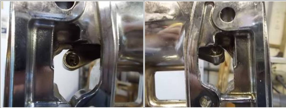
Check for wear at the side of the valve arms at the box 29)
