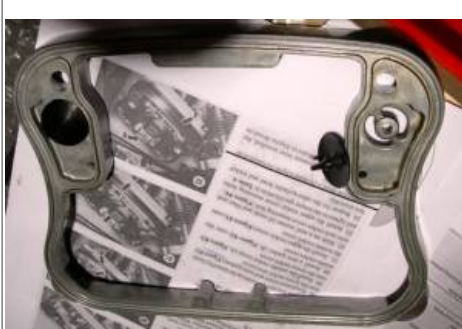
Umbrella Valve (only 1 installed per rocker box) 14) 15)
