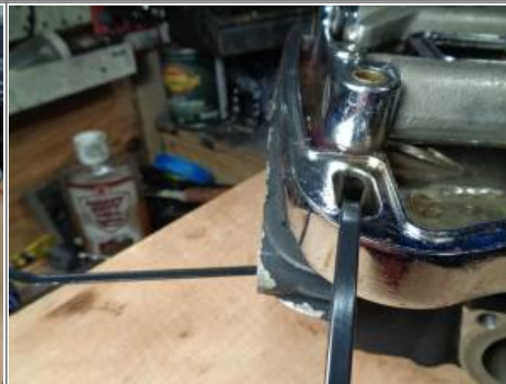
91-03 crankcase ventilation is done through the hole with the wire tie. 17)
