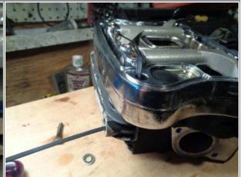
91-03 crankcase ventilation is done through the hole with the wire tie. 17)
