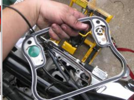
Umbrella Valve (only 1 installed per rocker box) 14) 15)
