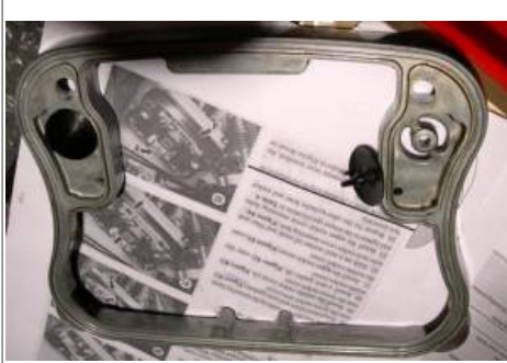
Umbrella Valve (only 1 installed per rocker box) 14) 15)
