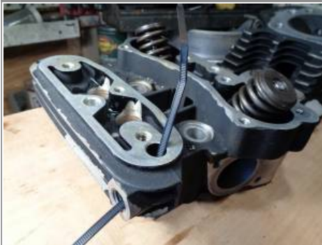
91-03 crankcase ventilation is done through the hole with the wire tie. 17)
