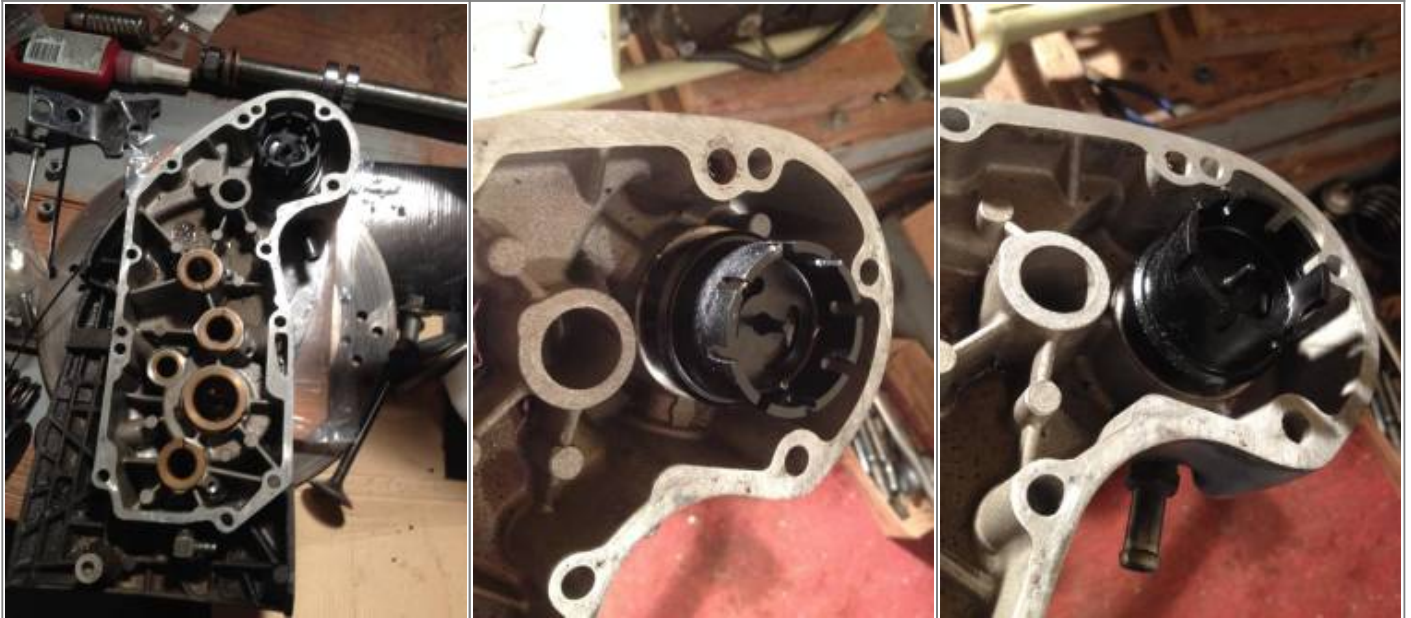
89 cam cover with breather baffle tube attached (it should be tight but still pull out) 8)
