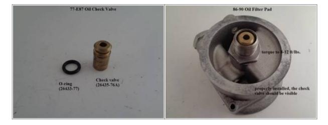
The check valve is not a pass through but instead a cartridge type one way check valve operated by a spring loaded cup against a seat pressing at 4-6 PSI. Oil pressure enters the center of the check valve, lifts the cup against its spring and exits the check valve by pushing around and past the cup and into the engine. At a point, the cup will float off it's seat up against the spring towards the end of it's travel.
