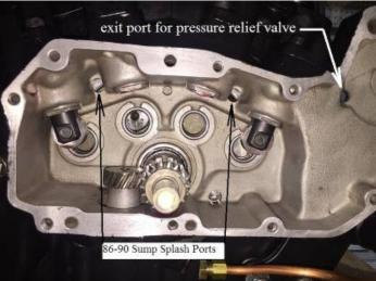
With the new Evolution engine in 1986, an oil pressure regulator (relief valve) was implemented to bleed off some of the oil when the pressure thru the filter became to high.
