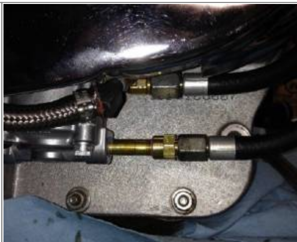
Alternate extension for the feed fitting 29) 30)
