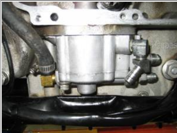
86-90 oil pump as installed 3)
