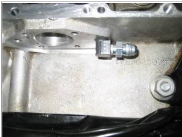
Oil entrance hole tapped with a 90° fitting installed 20)
