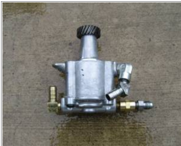
07 Pump feed side fitting with extension added 28)
