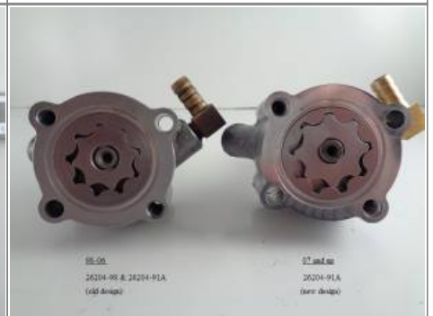
98 and 07 feed gerotors installed 24)
