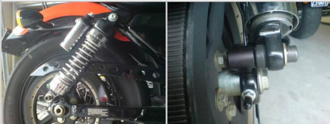
Shocks and lowering blocks installed <sup>2)</sup>
