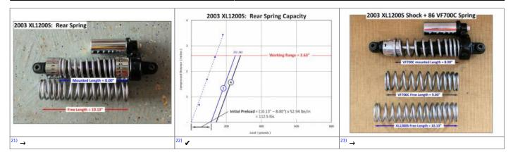
I wanted a different setup to handle the preload setup for the shocks with a coil over sleeve as I find these excellent to dial your suspension preload and top end right in. The problem is no one makes a coil over sleeve in that small of a diameter (~1.75") because there is no market for these small sleeves. I found the rear shock for a 2007 Victory Jackpot with a coil over sleeve that looked to be close to the size I needed.
