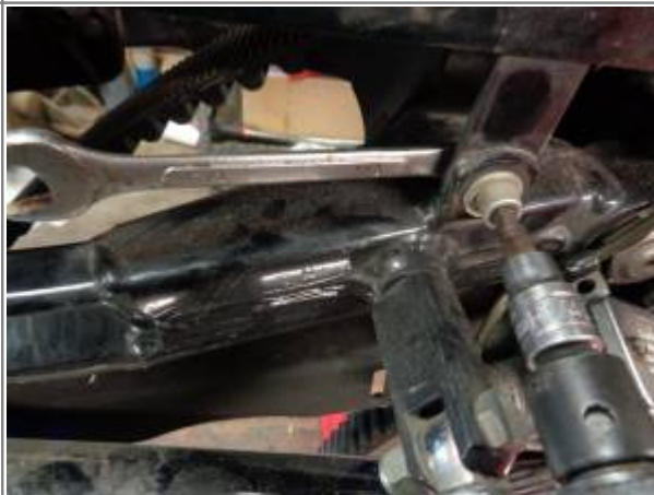
With the belt guard removed, the belt just slides around and out of the swingarm. 3)
