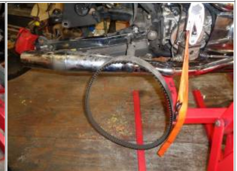
With the belt guard removed, the belt just slides around and out of the swingarm. 3)
