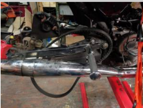
With the belt guard removed, the belt just slides around and out of the swingarm. 3)
