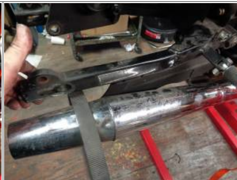
With the belt guard removed, the belt just slides around and out of the swingarm. 3)
