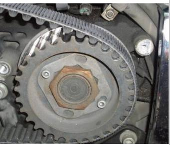
Pre-2004, on the outer flanged side, the center mounting splines are relatively flush with the flange face. But, on the engine side of the sprocket, the center mounting splines are recessed from the edge of the belt drive face. On 2004-later, the flange is on the engine side (with recessed splines there) and the mounting nut and lock plate are on the outer, flangeless, side.
