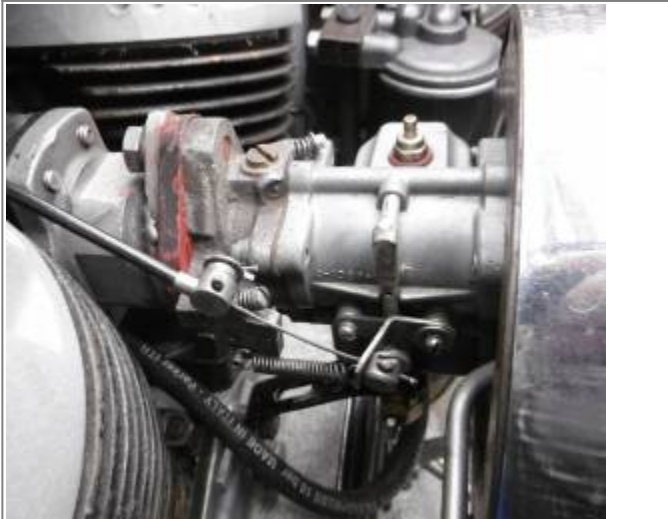
Linkage modified for usage with "snap" throttle 17)
