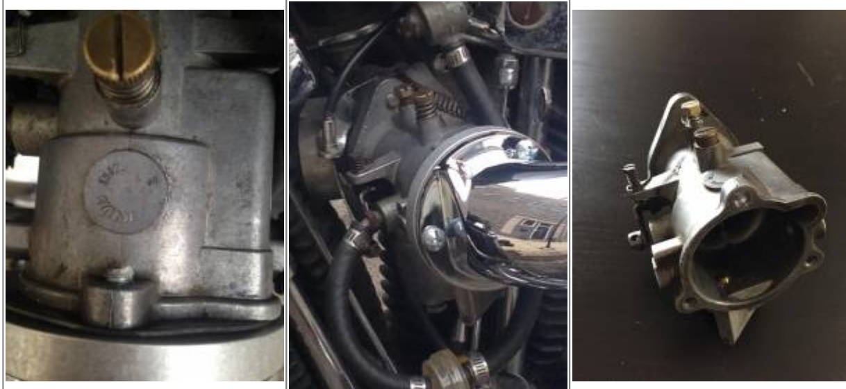
27152-71 (13479E) arbitrary 'E', fixed jet, 36mm 29)
