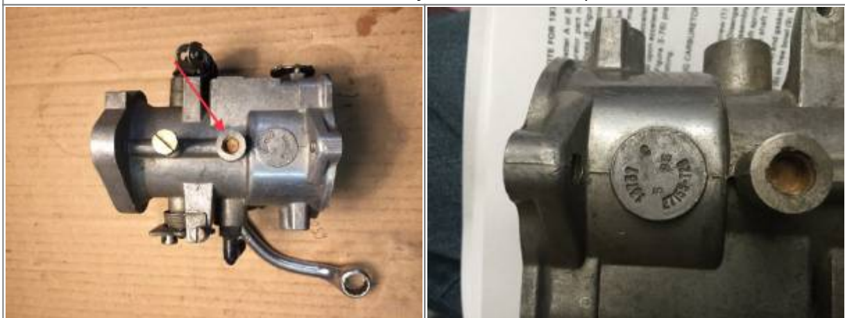
27155-72B (13731C), arbitrary 'C', venturi stamped 38mm 24)
