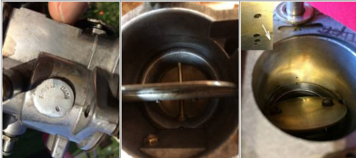
27155-72B (13731C), arbitrary 'C', venturi stamped 38mm 24)
