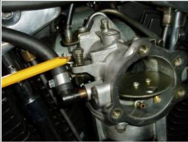
Throttle Stop Screw (idle speed adjuster): 23)
