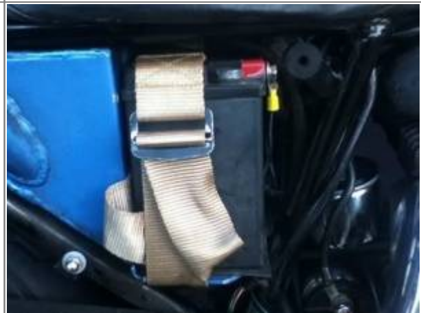
Possible temp fix for missing bracket 71)
