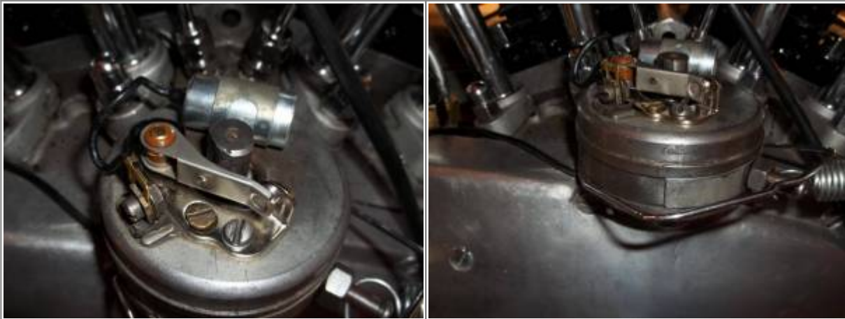
Single Point Circuit Breaker on a 57 XL 8)
