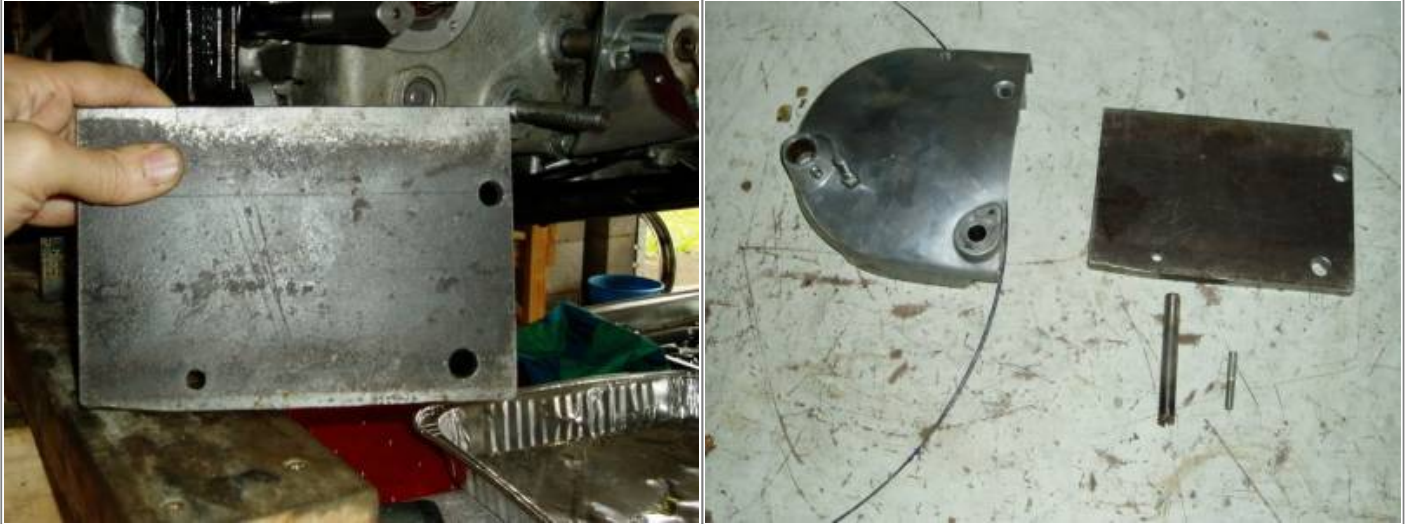
Drill jig made from a half-inch steel plate to guide the drill 4)
