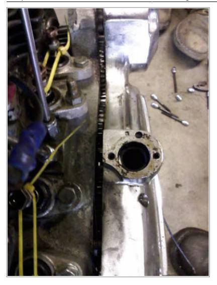
• Now look in the gap, and with a skinny screw driver, push all the cams back into the engine so that they won't come out with the cover.
