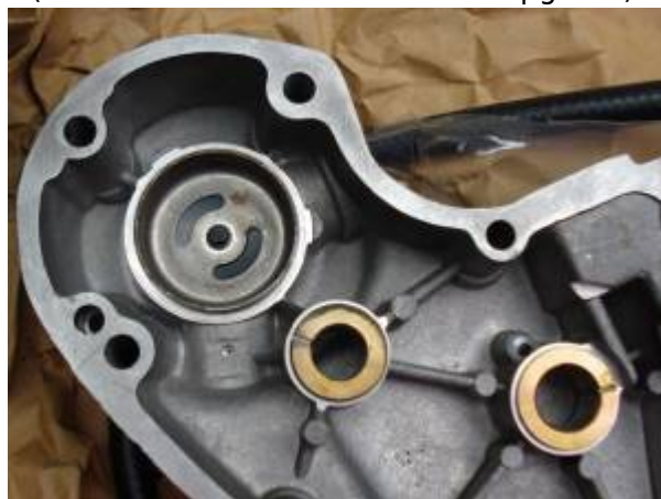
(Right) - 81 Cam Cover Breather Compartment (with the rubber umbrella valve upgrade). 24)
