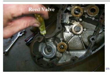
Here is the reed valve assembly front and back side.
