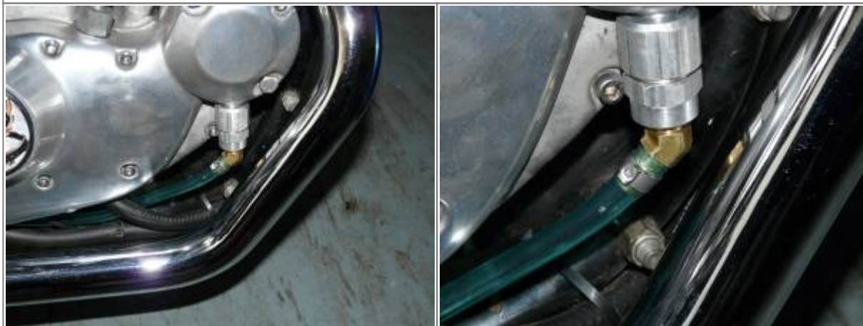
Stock tube removed, fitted with 1/8" 45 deg barb fitting. 23)
