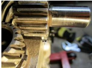
Pinion gear should be installed onto shaft so the outer face
