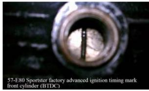
The flywheel needs to be positioned so the advance timing mark on the front cylinder is in the timing window.<sup>2)</sup> The single vertical line in most ironhead motors indicates the advance mark used for timing with a timing light.<sup>3)</sup> This line is also used for setting the breather and has nothing to do with pinion gear marks, cam marks or TDC of the pistons.
