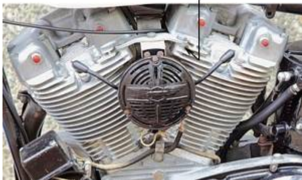
1960 XLCH Top Motor Mount (washer under head strap at each bolt, no washer under bolt head)
