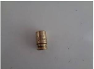
The check valve is not a pass through but instead a cartridge type one way check valve operated by a spring loaded cup against a seat pressing at 4-6 PSI. Oil pressure enters the center of the check valve, lifts the cup against its spring and exits the check valve by pushing around and past the cup and into the engine. At a point, the cup will float off it's seat up against the spring towards the end of it's travel.
