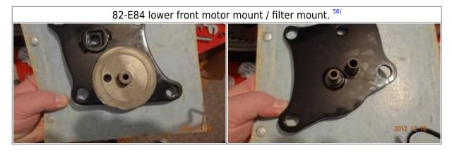
Oil filter mounting threads are M16 x 1.5mm.  $^{57)}$
