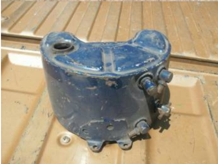
Aftermarket horseshoe tank (no drain): 16) 17)
