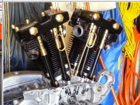
Brass oil lines on a 62 model 48)
