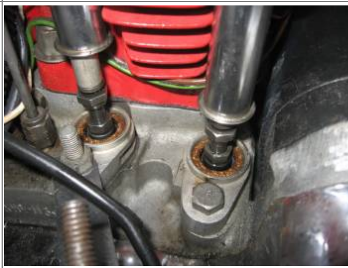
JIMS replacement tappet block with 1 straight and a couple spiral channels. 48)
