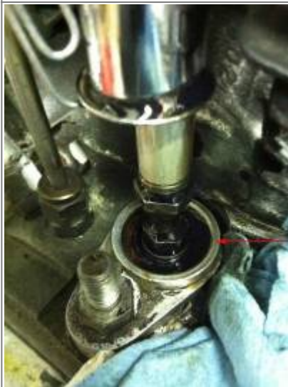
JIMS replacement tappet block with 1 straight and a couple spiral channels. 48)
