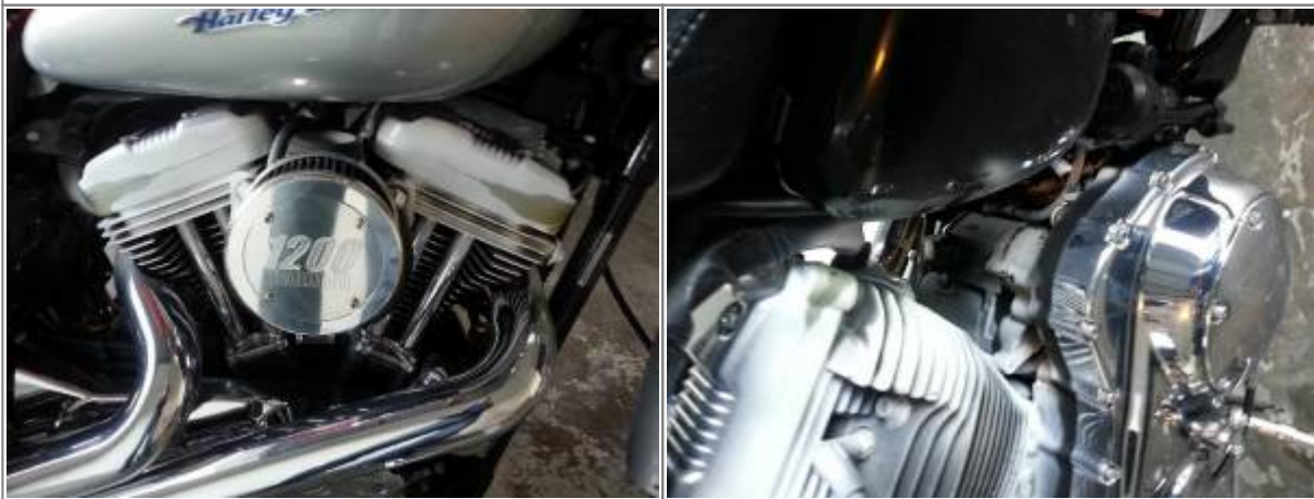
Rocker boxes sprayed with powder antiperspirant to detected oil leaks. 79)
