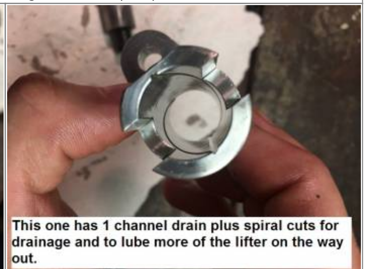
JIMS replacement tappet block with 1 straight and a couple spiral channels. 48)
