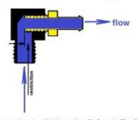
Make sure nipple fitting isn't installed deep enough to resrict oil flow.
