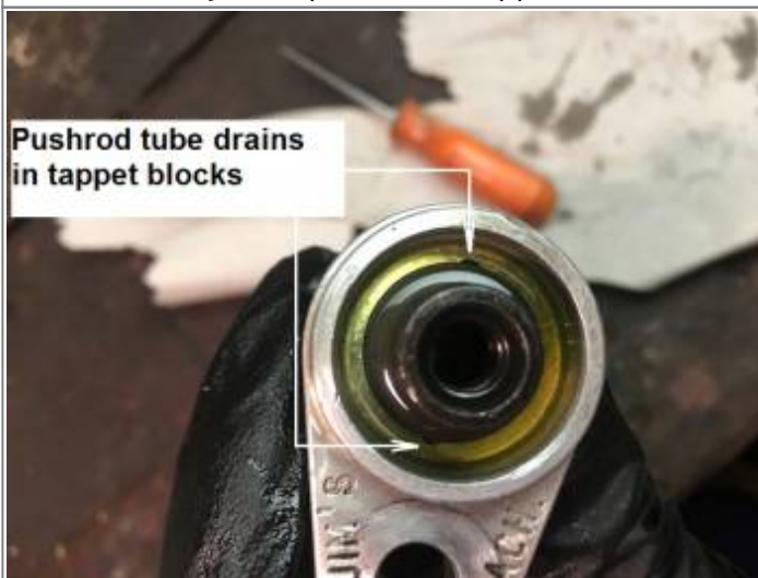
JIMS replacement tappet block with 1 straight and a couple spiral channels. 48)
