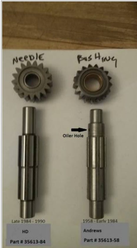
4 Speed Trans Countershaft comparison 166)
