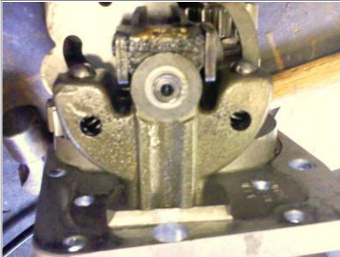
Next is the old Trock cast iron tower. By far the best shift fork control Never breaks, best of both worlds. 174)
