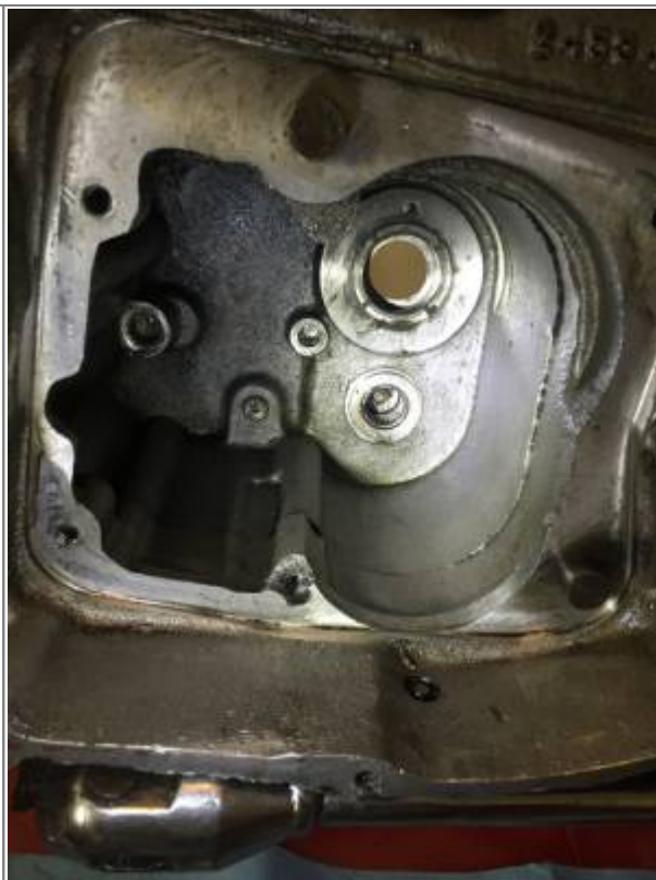
4 Speed housing inside 1977 XLCH case 176)
