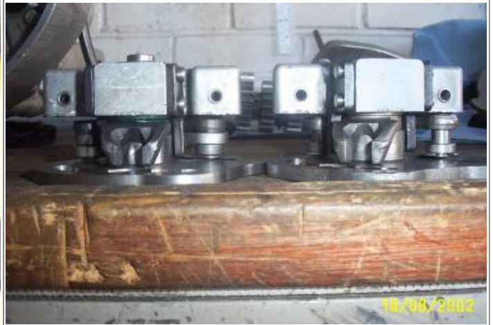
Left '72-'76 Shift Tower (taller shaft than on the right)
