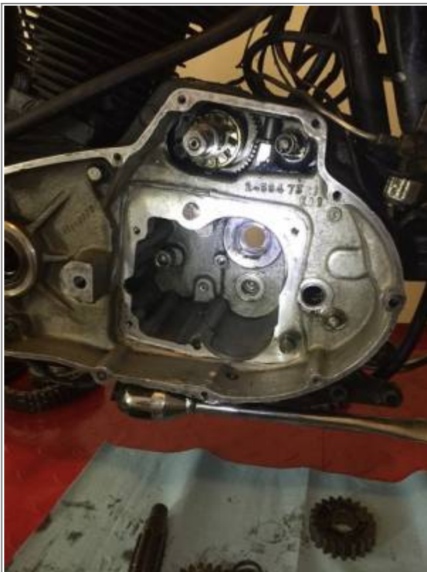
4 Speed housing inside 1977 XLCH case 176)
