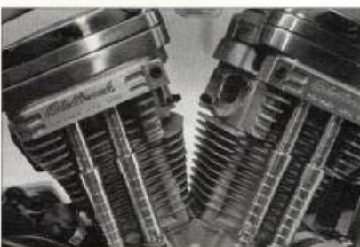
28 Place the stock center and new CCE finned upper rocker box into position, making sure the gaskets are properly aligned. Hand tighten the mounting screws and washers in a sequential pattern. Then torque them to 120 in-lb in the same sequential pattern.
