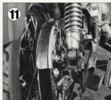
11 With the bike on its wheels, it's time to adjust the belt tension. This should be done with the bike resting on the kickstand, with the transmission in neutral, and no one sitting on the bike. The old chain adjusters are also used for the new belt drive. Each adjuster nut should be moved exactly the same number of turns as the other one. Remember, turning the adjuster clockwise will tighten the belt and counterclockwise will loosen it.
