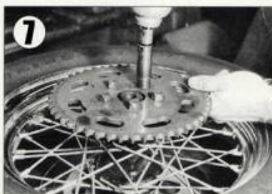
7 After you remove the rear wheel, unbolt the old sprocket.
