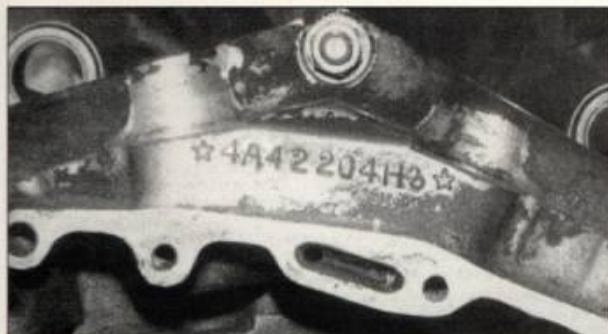
2 Here are the new style numbers which were used on 1970 to 1980 Ironheads. These also have a coding system. This number identifies the bike as a 1973 kick start 1000cc XLCH Sportster.
