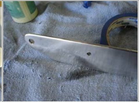
The bag mounting holes in the bracket were partially counter bored to allow clearance between the hardware and swingarm. 13)
