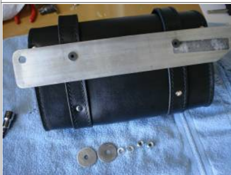
If after the bag gets broken in and it sort of flops over, you can add some metal flat stock inside the bag to keep it rigid. 17)
