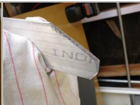
Edges rounded with a file, bracket wet sanded with 320/400/1500 grit paper respectively and then hand polished. 10)
