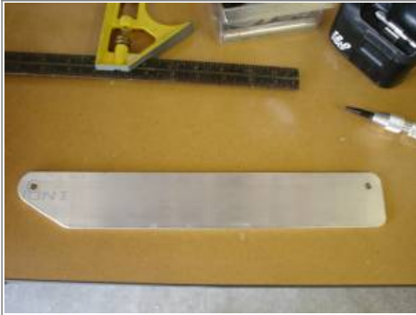
Final fitting to mark a hole on the rear side at the swingarm. 11)
