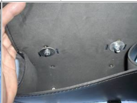
If after the bag gets broken in and it sort of flops over, you can add some metal flat stock inside the bag to keep it rigid. 17)
