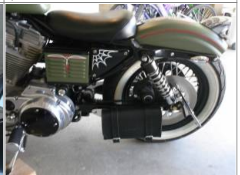
Bag mounted with chrome buttonheads, spacers and Loc-tite. 16)
