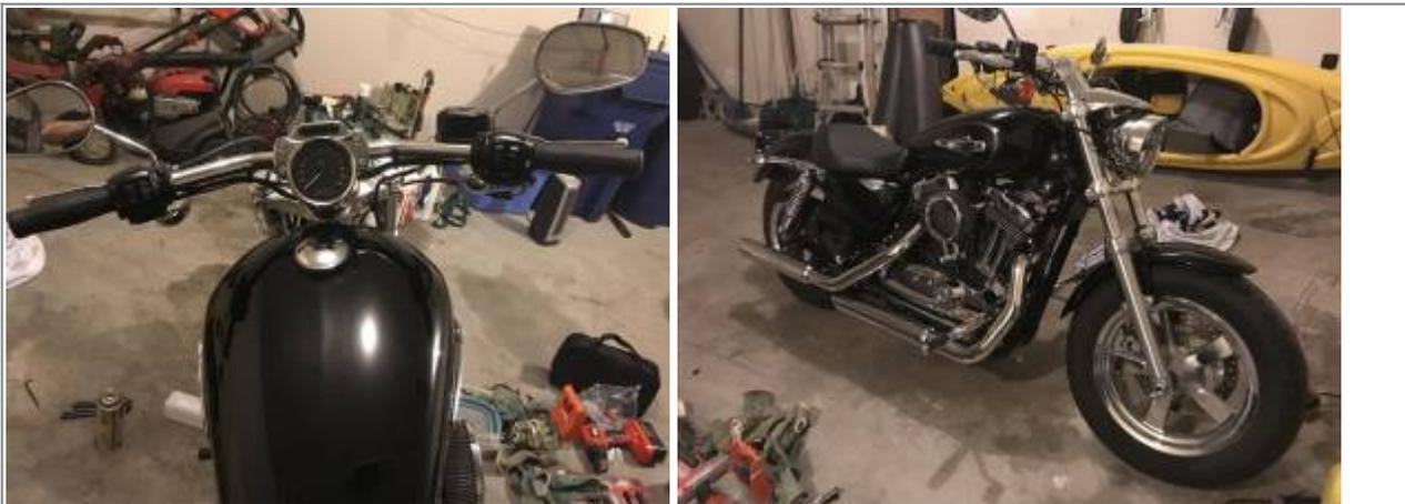
1" Drag Bars w/ stock risers and cables on a 2014 XL1200C - 30" wide, 6" pullback, 8" center. <sup>1)</sup>
