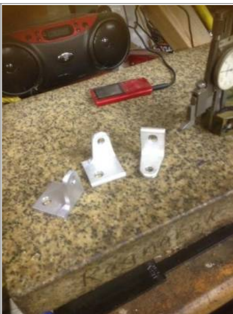
Fabricate some 1/2" 6061 aluminum brackets 3)
