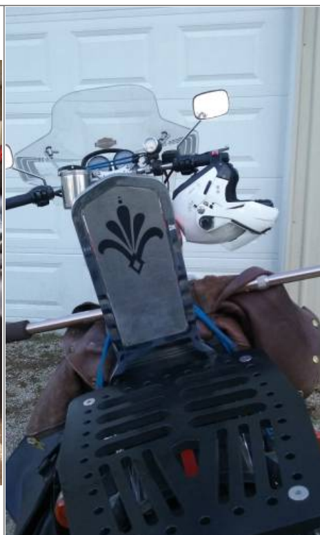
Add an aluminum 6061 insert into the sissybar (laser etched) to match the rack 9)
