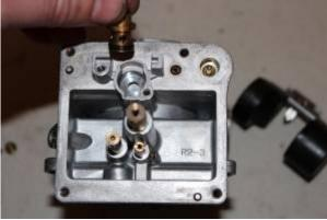
Unscrew and remove the main jet, main jet extender and the needle jet underneath should come out with a tap, as well.
