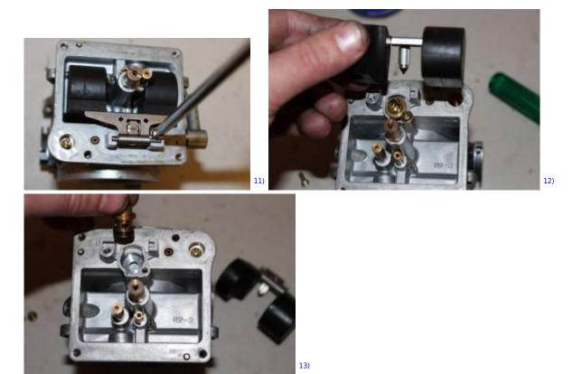
Unscrew and remove the main jet, main jet extender and the needle jet underneath should come out with a tap, as well.
