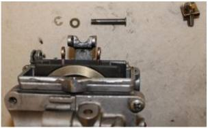
You can then remove the 3 remaining screws to remove the back carb body and 4 screws to remove the float bowl.
