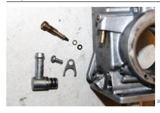
Remove the float assembly by unscrewing the float pin screw. The plunger of the needle valve assembly will come out with it.
