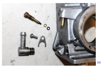
Remove the float assembly by unscrewing the float pin screw. The plunger of the needle valve assembly will come out with it.
