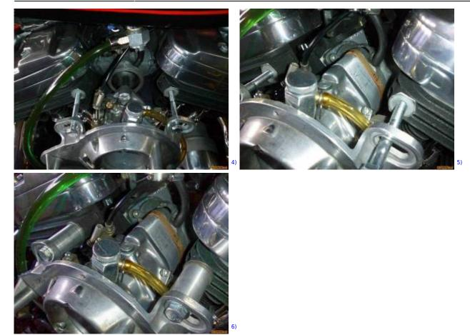
This is how far the carb sticks out with the spacer installed.
