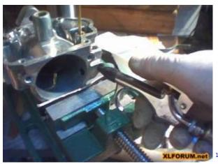
I decided to skip option 6. I don't think it's necessary for a 1200 motor if you're not revving to 7500 RPM. Now moving on to the float bowl. We have to install the fuel nipple that supplies fuel to the ThunderJet.
