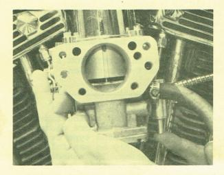
After carburetor is installed on manifold, with leveling bracket in position level the carburetor and tighten the manifold clamps securely. Install the Piston & Dome carefully as the tapered needle will bend if abused. Secure the dome and check for free piston up and down movement. If piston is sticky, loosen dome screws and re-locate until piston moves free. Attach Fuel line to ½" fitting. Turn fuel on.
