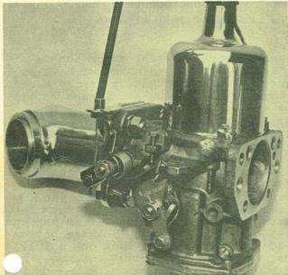
Remove dome and piston. Install the "ELIMINATOR II" body (shown) to the manifold with the hardware supplied. The standard bracket for cable holder mounts on the outside top of manifold. (shown in Fig 7). There is a cable holder on top of the bracket. 1973 & later models:
