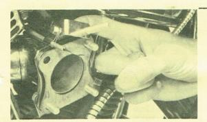
Install the manifold in the usual manner. We advise using teflon tape to cover the "O" rings before clamping. 1981 and up use band type seals. Install clamps lightly as manifold will require leveling. The standard leveling bracket is mounted from the center case bolt of the engine to the bottom left manifold hole, for later models mount in same position as stock mounted bracket.
