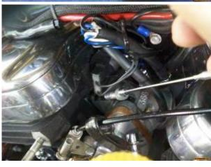
Now tighten the 4 intake manifold bolts. Basically you tighten the bolts till the flanges bottom out to the heads. Torque spec is 6-10 ft lbs.
