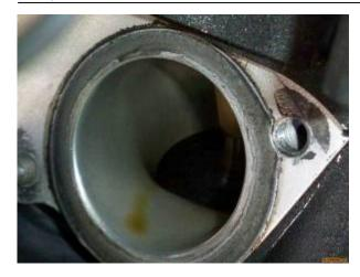
Before installing the intake assembly, make sure the flanges are turned the correct way.
