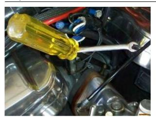
With all 4 of the intake manifold bolts are removed, then remove the 2 bolts that hold the air cleaner back plate to the heads. <sup>3)</sup>
