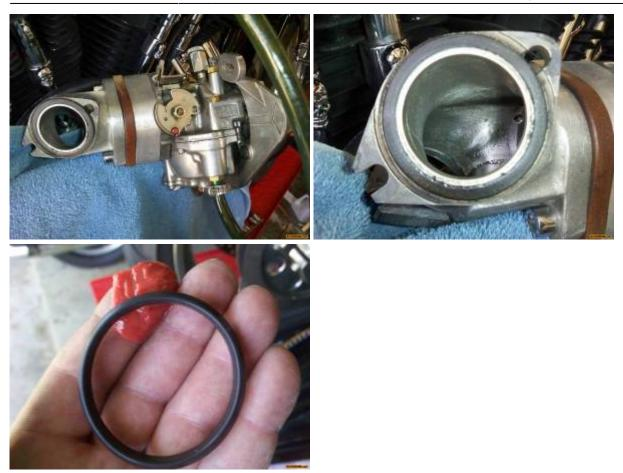
Install the seals. Don't forget to clean where the seal fits to the head. 5)
