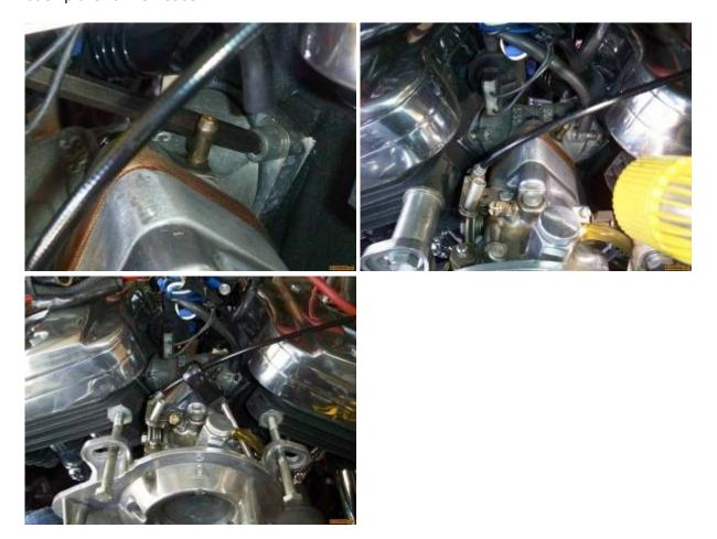
Now you should be able to remove the entire intake manifold, carb, back plate assembly. The throttle cable was left on below since the carb will not be serviced here but just the manifold seals. Applying some grease to the seals prior to installation will help keep down air leaks later. <sup>4)</sup>
