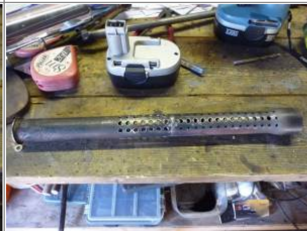
Holes in the baffle partially drilled out. 24)
