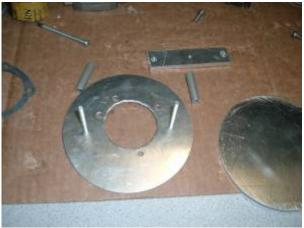
Drill two holes in the plate for dowels (spacers) for the front cover (also created from tracing the filter). Cut a mounting bracket (this one is 1/4" thick) to mount across the dowels and tap the bracket for the size mounting bolts you choose.
