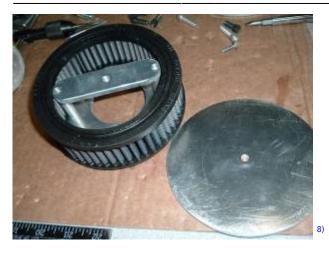
Make sure you test fit along the way as it's being built. The bolts and spacers here made contact with the carb bracket.
