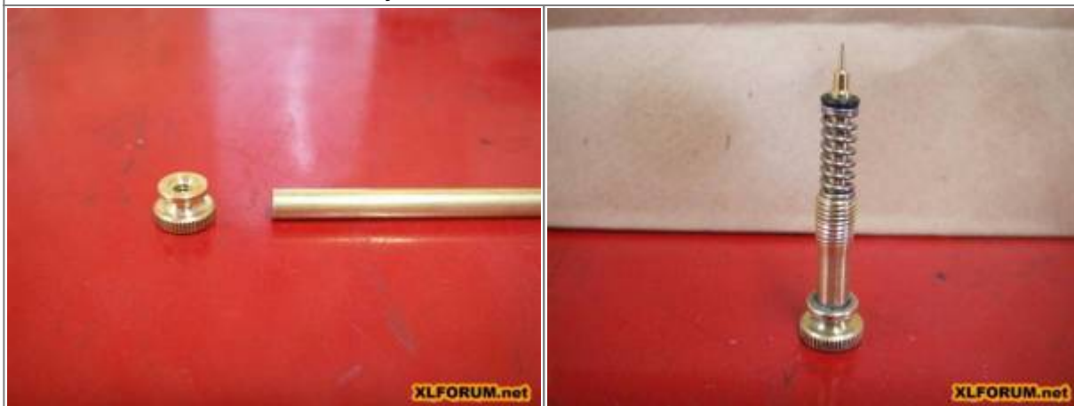
Factory idle mixture screw extended. 20)
