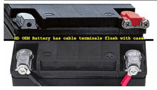
But almost all aftermarket batteries have a recessed cable connection. It is not flush with the battery case, but rather is recessed about 3/16' of an inch. However, most batteries also come with spacers that allow the HD-style flush mounting of the cables.
