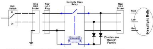
Set Headlight Hi/Lo switch Hi - Then Key switch to ON Start Bike - Relay open contacts keep headlight OFF After starting, set headlight switch to Lo Relay will be latched ON and headlight will operate as normal in either Lo or Hi position until key switch is turned OFF
