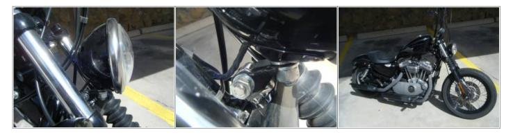
The bottom of the mount was tapped for a 1/4" bolt to run through the tree.
