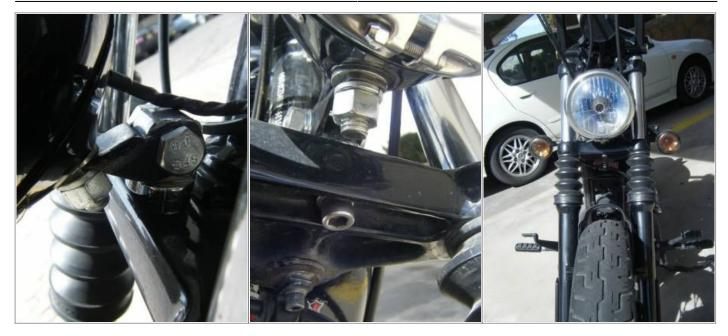
The 2 piece mounts were welded together with a mig welder using flux core wire. Here are some drawings of the mounting bracket (dimensions not to scale). <sup>3)</sup>
