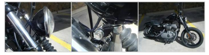
The bottom of the mount was tapped for a 1/4" bolt to run through the tree. The bolt going through both mount halves is 1/2".
