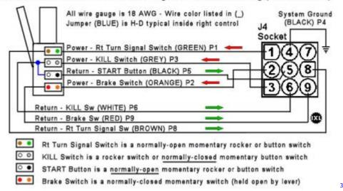
Note that on most Sportsters, all the way up thru 2013, the wiring configuration is functionally the same as above (with only some minor wire color variations - or those noted in the TH Install Manual). The BLUE jumper wire shown in the diagram between the RUN/STOP Switch and the Starter Button is typically internal to the RH Switch Housing.
