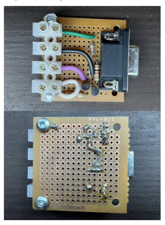
If anyone wants to make the same, here is a hand drawing of the layout. It is arranged so no jumper wires are needed on the underside. All components that need connections are placed with adjacent pins so they can just use a solder bridge between them. In the below drawing the blue pen lines are solder bridges between component pins.
