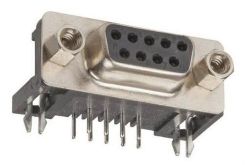
The pins don't all line up the same as the PC board that I used so I broke off pins 1, and 6-9 which aren't used anyway.
